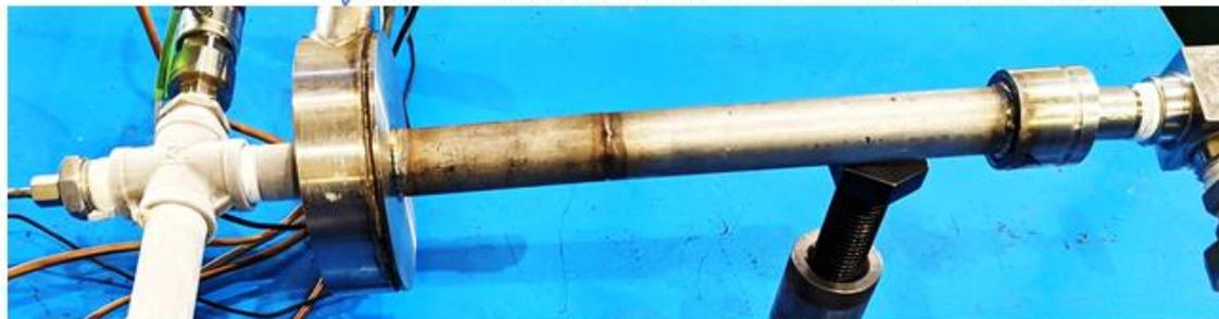
(5) Type-A Fin, Pitch = 30 mm,  $\Phi = 10$  mm,  $L_c = 108$  mm,  $L_{fin} = 200$  mm,  $L_h = 0$  mm,  $L/D = 10.0$
