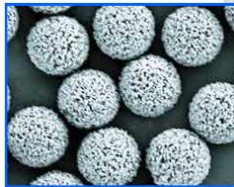
Chromatographic beads (Porous particle)
